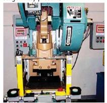
All machines consist of three fundamental areas; the point of operation, the power transmission device, and the operating controls. Despite all machines having the same basic components, their safeguarding needs widely differ due to varying physical characteristics and operator involvement.
