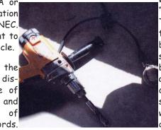
manager of their Regulatory and Compliance Division, and he stated: "Makita does not permit the mounting of a three-prong, grounded type plug on a double-insulated tool". He further explained that NEC 406.9 (E) states "Grounding-type attachment plugs shall be used only with a cord having an equipment grounding conductor. Since a double-insulated tool is not provided with an equipment grounding conductor the use of a grounding type plug on the tool is prohibited".
